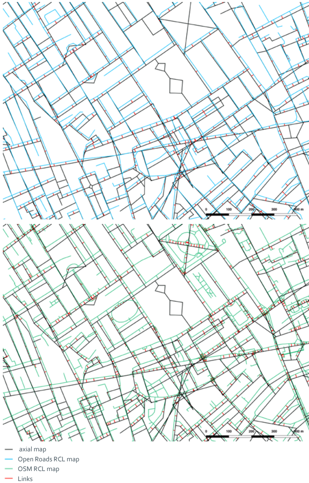
Figure 1 - Each RCL segment is linked to one or many axial lines
